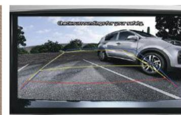
**Parking guide system** Steering wheel mounted angle sensors and a rear-view camera indicate the projected trajectory of your vehicle for added safety.
