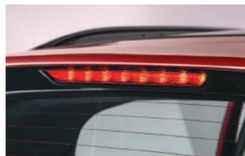
**High Mounted Stop Lamp** Other vehicles need to vividly see you stopping on the road, thanks to the high mounted LED stop lamp integrated in the rear spoiler.
