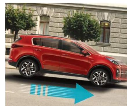
**Downhill Brake Control (DBC)** Sportage's DBC supports the driver driving down a steep hill without the driver depressing the brake pedal. It slows down the vehicle and lets the driver concentrate on steering the vehicle.
