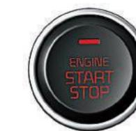
**Button start / stop** For convenience and safety, you don't have to take the key fob out of your pocket when you're locking or unlocking the door, starting the engine or disengaging the immobilizer.
