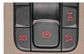
**Electronic Parking Brake (EPB)** State-of-the-art switch design for activating the parking brake provides added convenience and saves space.
