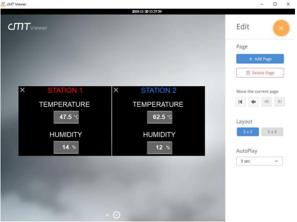
Note: To show real-time data for the project of a cMT-FHDX like below, you must enable Monitor Mode in Easybuilder pro and create a screen for visualization. Here are steps to configure.
