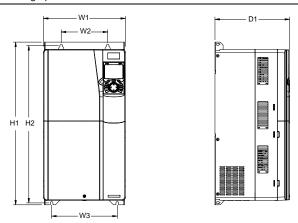
Figure C.5 045G/055P-075/090P wall-mounting diagram
