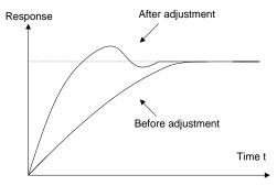
**Control long-term vibration:** If the cycle of periodic vibration is longer than the set value of integral time (Ti), it indicates the integral action is too strong, prolong the integral time (Ti) to control vibration.
