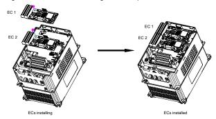
Figure A.2 VFD of 5.5 kW or lower with expansion cards installed Expansion card installation process:
