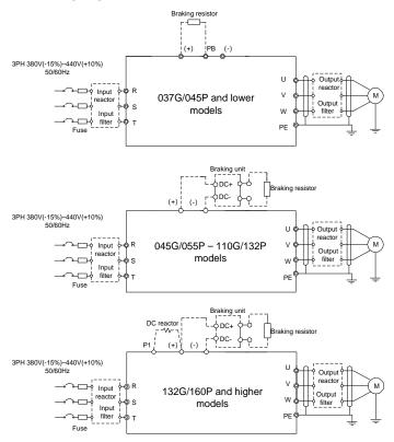
Figure 4.7 Main circuit wiring diagram
