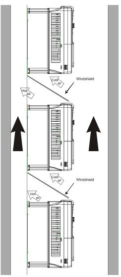
Figure 4.5 Vertical installation
