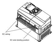
Figure A.5 Expansion card wiring
