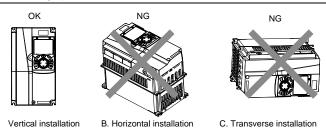
Figure 4.1 Installation direction of the VFD
