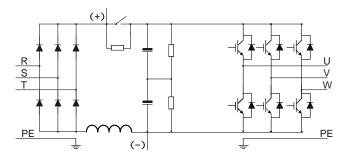
Figure 3.3 Main circuit diagram for 045G/055P-110G/132P
