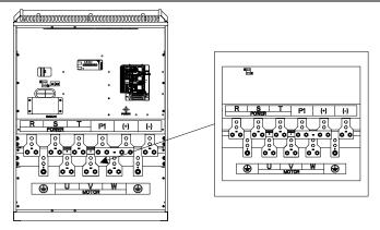
Figure 4.12 Main circuit terminal diagram for 220G/250P-315G/355P models
