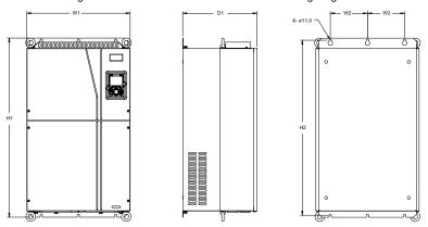
Figure C.7 132G/160P-200G/220P wall-mounting diagram
