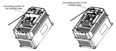
Figure A.4 Expansion card grounding diagram
