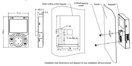
Figure C.1 Keypad structure diagram
