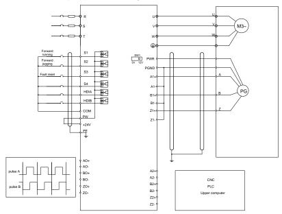
The following figure shows the external wiring of the expansion card used in combination with a push-pull encoder.
