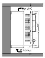
Figure 4.4 Parallel installation
