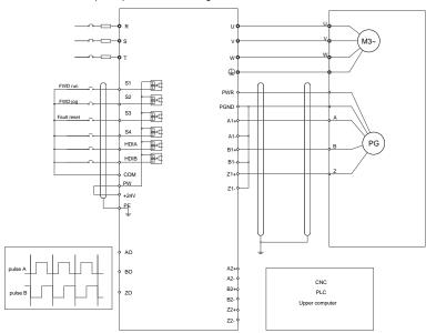
The following figure shows the external wiring of the PG card when it is used in combination with a push-pull encoder.
