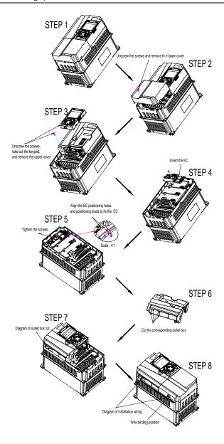
Figure A.3 Expansion card installation process diagram
