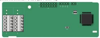
The DIP switch SW1 is used to set the voltage class (5 V or 12 V) of the power supply of the encoder. The DIP switch can be operated with an auxiliary tool.
