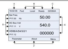
Figure 5.2 Main interface of LCD
