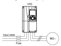
Figure 4.19 Fuse configuration
