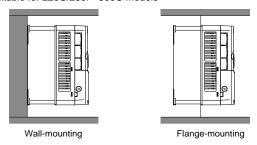
Figure 4.2 Installation mode
