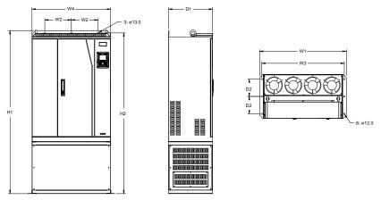
Figure C.12 220G/250P-315G/355P floor installation diagram
