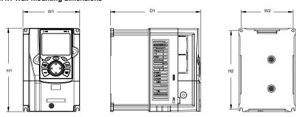
Figure C.4 1R5G/2R2P-037G/045P wall-mounting diagram
