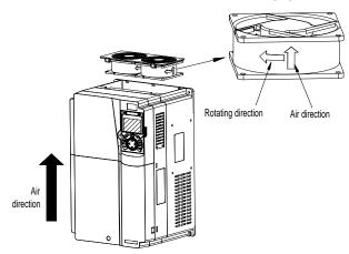
Figure 8.1 Fan maintenance for 7R5G/011P and higher models
