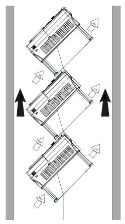
Figure 4.6 Tilted installation
