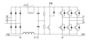
Figure 3.2 Main circuit diagram for 018G/022P-037G/045P
