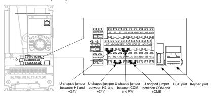
Figure 4.16 Position of U-type short connector
