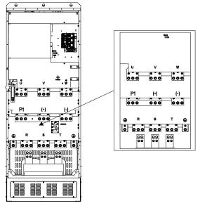
Figure 4.13 Main circuit terminal diagram for 355G/400P-500G models
