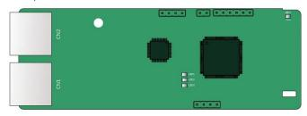
The communication port adopts standard dual RJ45 interfaces, and the two RJ45 interfaces are not distinguished from each other and can be interchangeably inserted.
