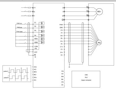
The following figure shows the external wiring of the PG card when it is used in combination with an encoder with CD signals.
