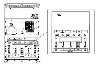
Figure 4.11 Main circuit terminal diagram for 132G/160P-200G/220P models
