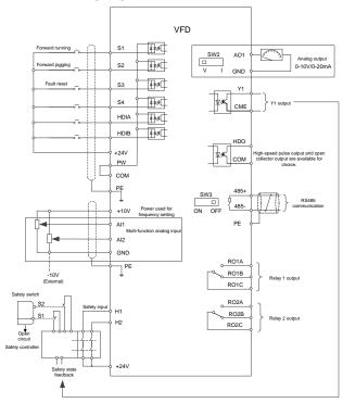
Figure 4.15 Control circuit wiring diagram
