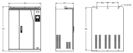
Figure C.8 220G/250P-315G/350P wall-mounting diagram
