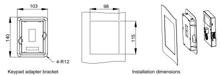
Figure C.2 1R5G/2R2P-500G keypad installation bracket (optional)
