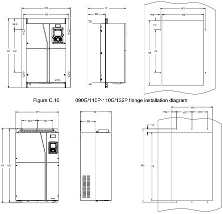
Figure C.11 132G/160P-200G/220P flange installation diagram
