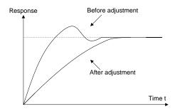
**Stabilize the feedback value as fast as possible:** when overshoot occurred, shorten integral time (Ti) and prolong derivative time (Td) to stabilize control as fast as possible.
