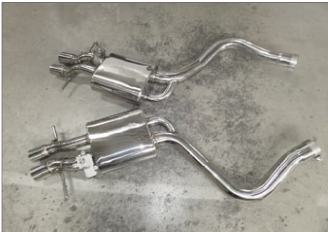
Mufflers 22M 221 009 set - left & right with throttle control
