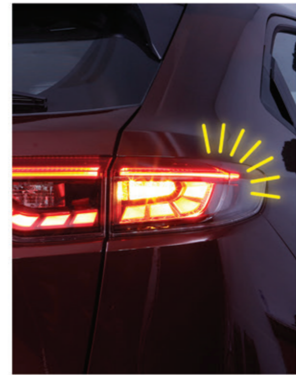
Emergency Stop Light
