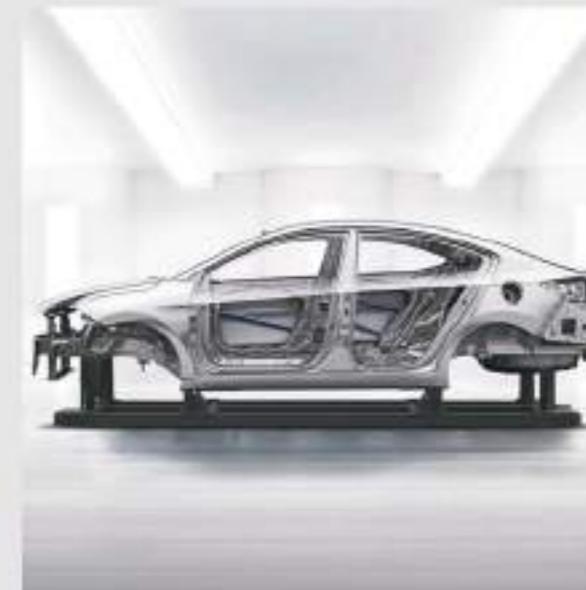
High Strength Steel Extended application of Ultra High Tension Steel Plate reinforces chassis rigidity.
