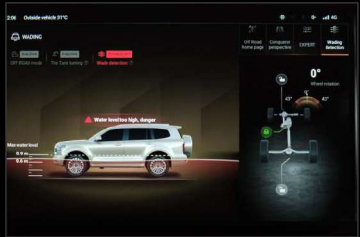
Wading Depth Detection Water depth detection system
