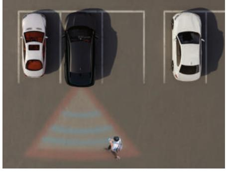
**Rear View Monitor with Dynamic Guidelines**A parking safety features that displays the rear view with parking guidelines using the rear view camera. It provides a rear top view for parking and trailer hooking and offers a continuous rear view driving for enhanced safety.
