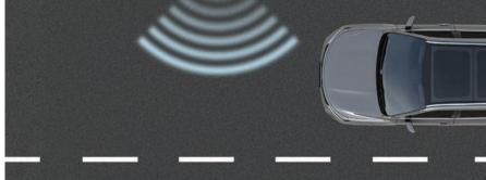
Safe Exit Assist (SEA) A driving safety function that provides a warning and assistance when a vehicle is approaching from the rear-side while someone is getting out of the vehicle.
