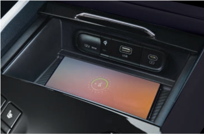
Wireless Charging Tray Fast and convenient wireless charger compatible with most smartphones for seamless charging.
