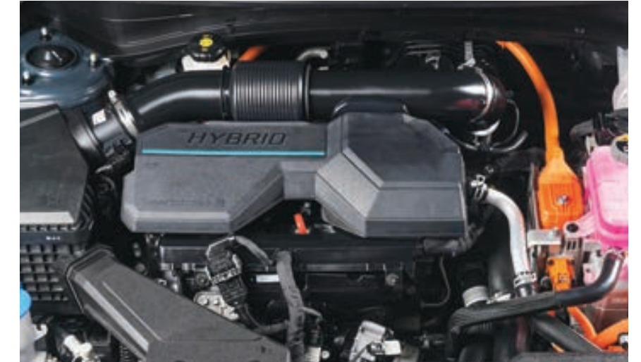
SmartStream G1.6T-GDI HEV Engine Maximum Power: 177 hp Maximum Torque: 265 Nm Motor Maximum Power: 59 hp Maximum Torque: 265 Nm Combined Maximum Power: 227 hp Maximum Torque: 350 Nm Transmission Speed: 6AT
