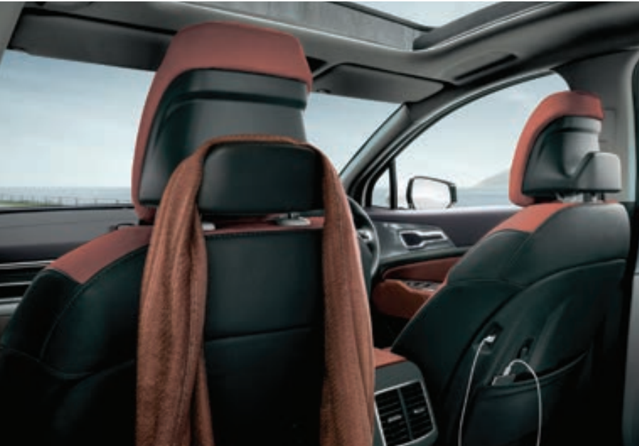
Headrest Hanger / USB Ports on Seatbacks The backs of the front headrests include built-in, shape-preserving coat hangers. Rear seat passengers will find convenient USB-C charging ports in the seatbacks ahead of them.
