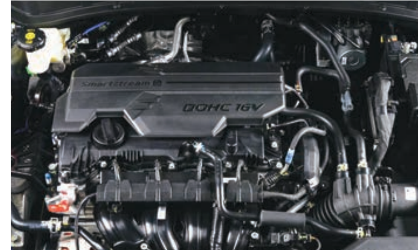
SmartStream G2.0 Maximum Power: 154 hp Maximum Torque: 192 Nm Transmission Speed: 6AT
