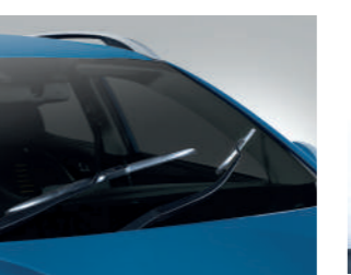
Aero Blade Wipers: Aerodynamic wiper blades maintain contact with the windshield, even at high speeds.
