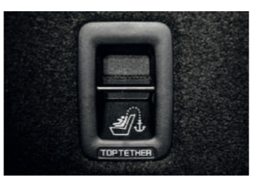
ISO Child Anchor: Keep your child safely and securely seated by strapping their seat to the special metal anchors in the vehicle.
