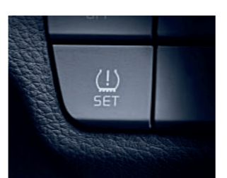
Tire Pressure Monitoring System (TPMS): Tire Pressure Monitoring System (TPMS) in your Stonic is designed to alert you of a change in tire pressure that could put you at risk.
