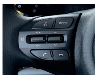
Steering Switches: Fingertip control of the sound system means you will never be distracted from the road ahead.
