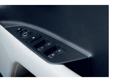
Power Windows: Power window controls for the rear doors give rear-seat passengers control over how much or little air to let in.
