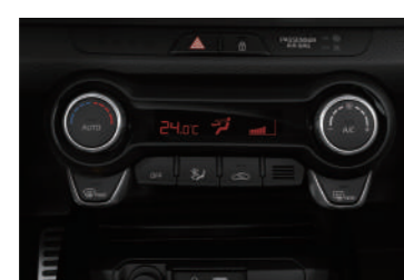
Auto Climate Control: Auto temperature control lets you select a desired temperature for the system to maintain. A digital readout displays temperature and settings.
