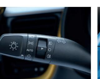
Auto Light Control: The headlamps are engineered to respond smartly to external light and adjust to its levels for better driving facilitation in the night time.
